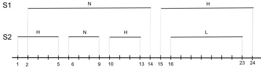
Fig. 3. Example of MSS with two variables measured over 24 time units. The values of S1 and S2 are discretized as low (L), normal (N) or high (H) and the sequence is represented as a series of state intervals  $Z = (E_1 = (S2, H, 1, 5), E_2 = (S2, N, 2, 14), E_3 = (S2, N, 6, 9), E_4 = (S2, H, 10, 13), E_5 = (S1, H, 15, 24), E_6 = (S2, L, 16, 23))$
