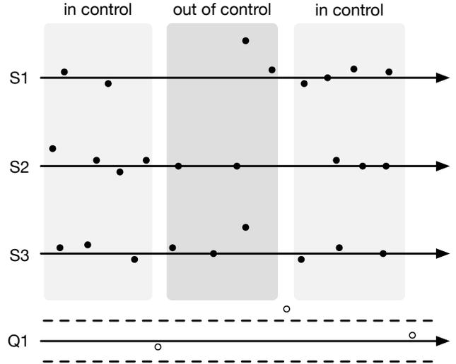
Fig. 2. An example of samples for the three output quality measurements. The quality metric determines the label (in control or out of control).
