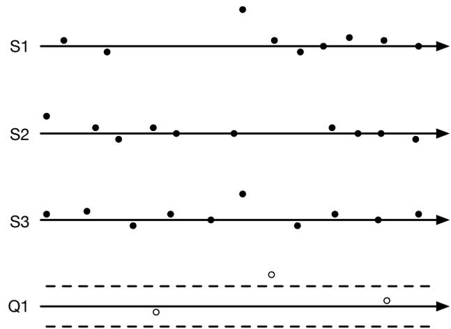
Fig. 1. An example of three operating conditions and one quality metric data over time. For each parameter, the intervals between measurements are irregular, and not necessarily aligned with the other parameters. The dashed lines illustrate the specification limits for the quality metric.
