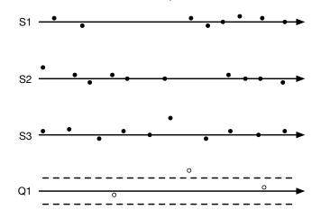
Fig. 1. An example of three operating conditions and one quality metric data over time. For each parameter, the intervals between measurements are irregular, and not necessarily aligned with the other parameters. The dashed lines illustrate the specification limits for the quality metric.
